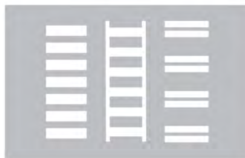
Typical crosswalk markings: Continental, Ladder, Staggered Continental (Credit: Michele Weisbart) Continental striping (far left)
